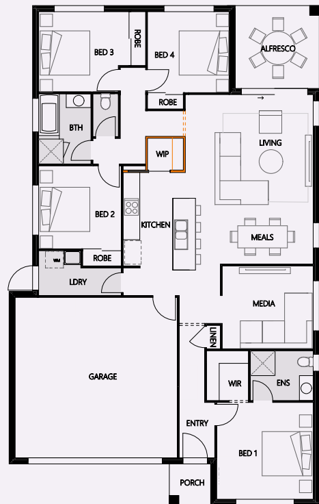
WALK IN PANTRY & BENCHTOP UPGRADE Remove cupboard pantry for 840mm of extra bench space + 720mm cavity slider + hamper
